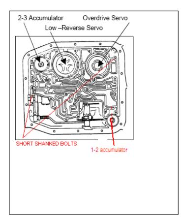
Note servo in diagram. From under car press up on the front servo just enough to take pressure off. With two small screwdrivers, or seal/gasket picks, remove the snapring. Release the jack slowly.
